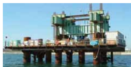
Photo 4 Static loading test
