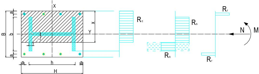
$$N_{sy} = R_s A_s - 4R_s T \left( \frac{B+b}{2} - x \right)$$
