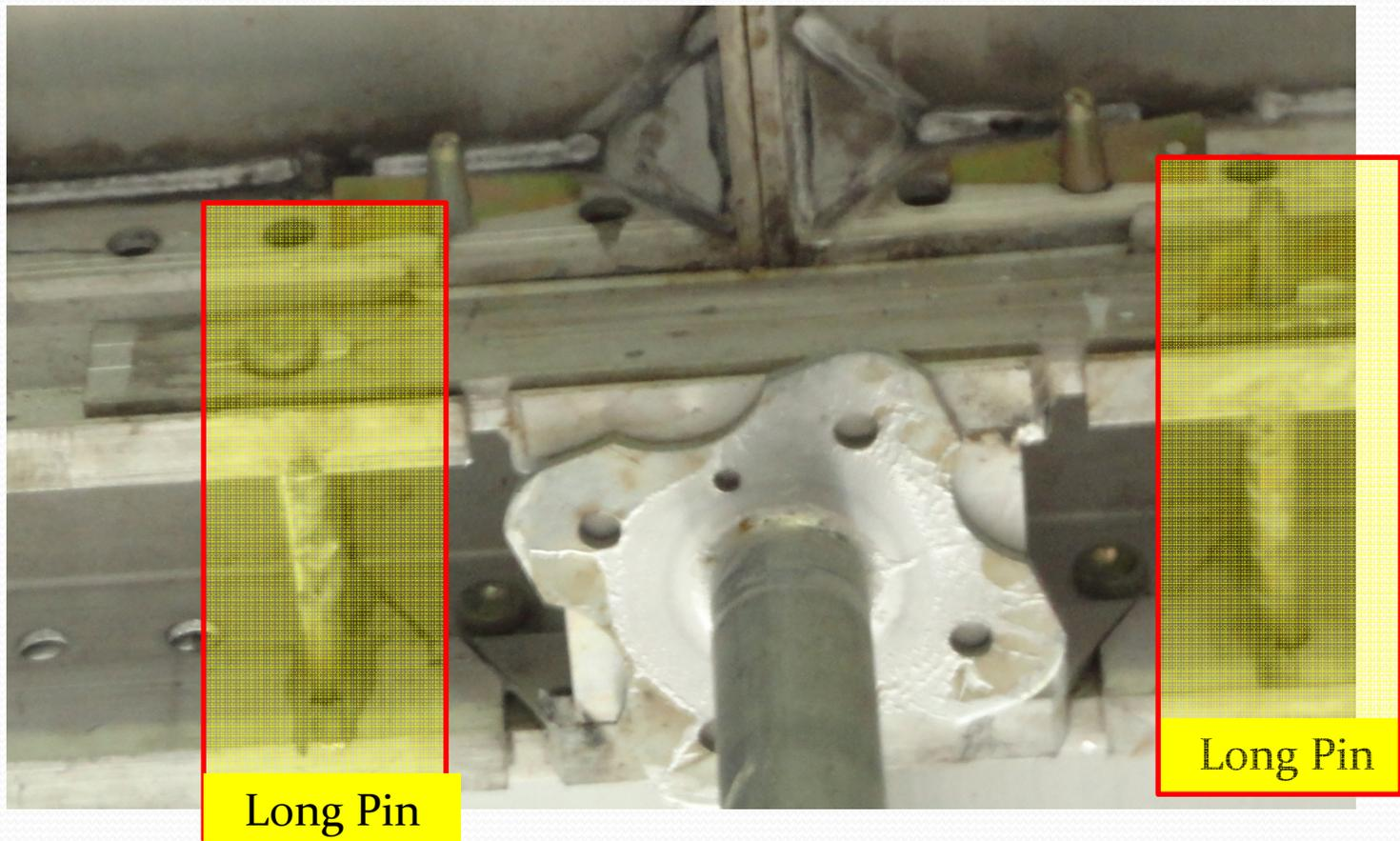
For connecting Joint bar & Prop head
