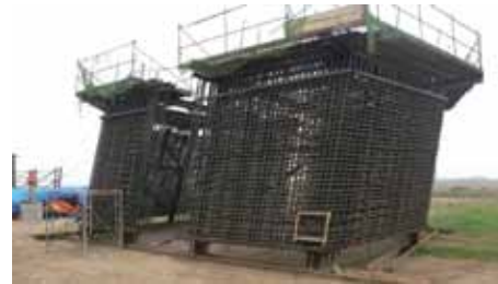
Photo 8 Full-scale model prepared to examine installation of reinforcing bar cage for main tower bottom section
